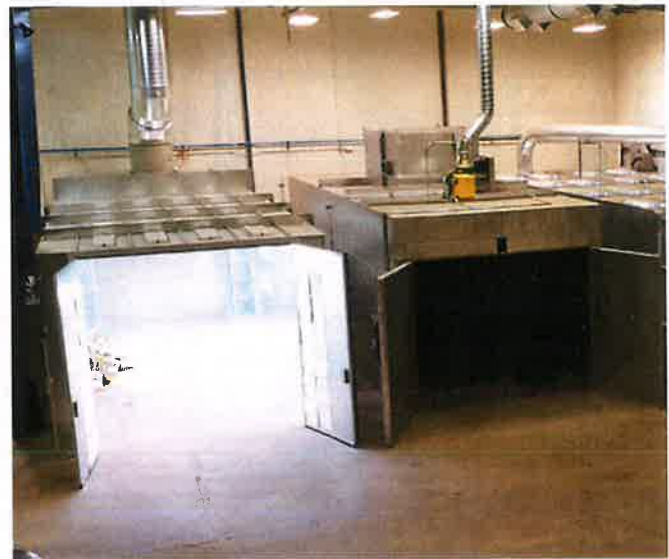
Besides the sheer weight of large parts, there are also inefficiencies that arise from using such a large oven for curing.
