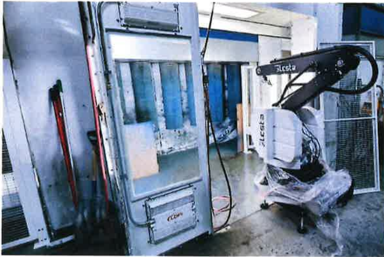
Painter powder coats a rack, recording his motions, which this robot can then repeat for the rest of the rack of parts.
